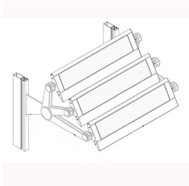
**LOUVER CROSS SECTION WITH PHOTOVOLTAIC PANEL**
