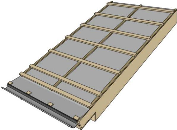
The battens, counter battens and wedges are installed.
