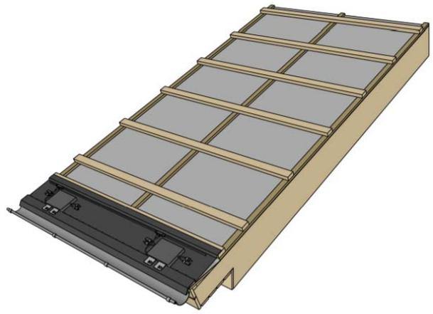
The inverter drawer and then the micro-inverters are installed.
